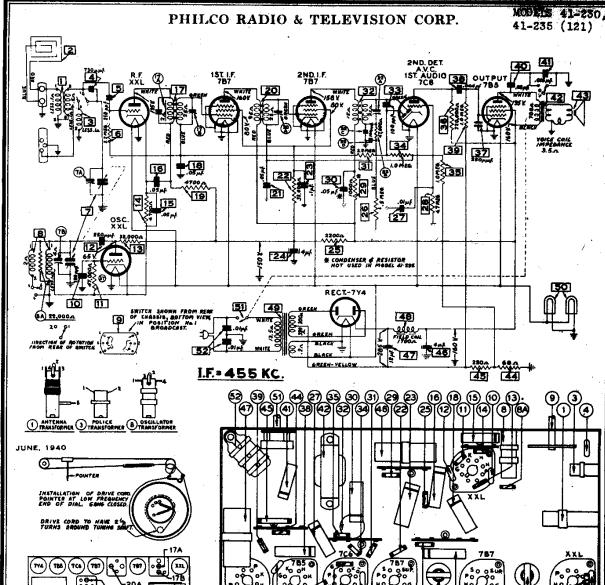
When aligning the R. F. padders a loop is made from a few turns of wire and connected to the signal generator output terminals; the signal generator is then placed close to the loop of the radio.
